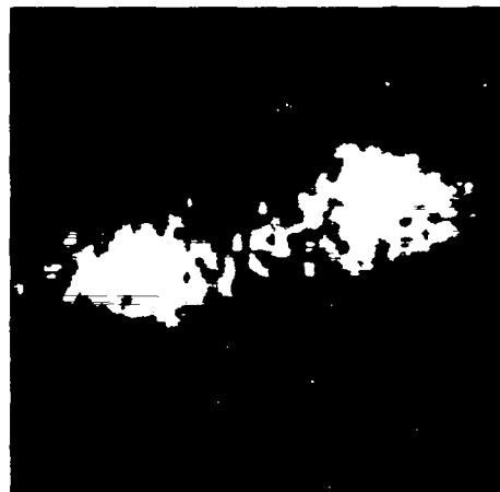
Fig. 76 X-ray image of two 6-μm holes 100 μm apart.
